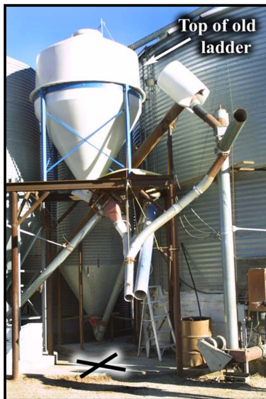
Photo 2 – Side view of old grain bin ladder and concrete pad where the victim fell.
